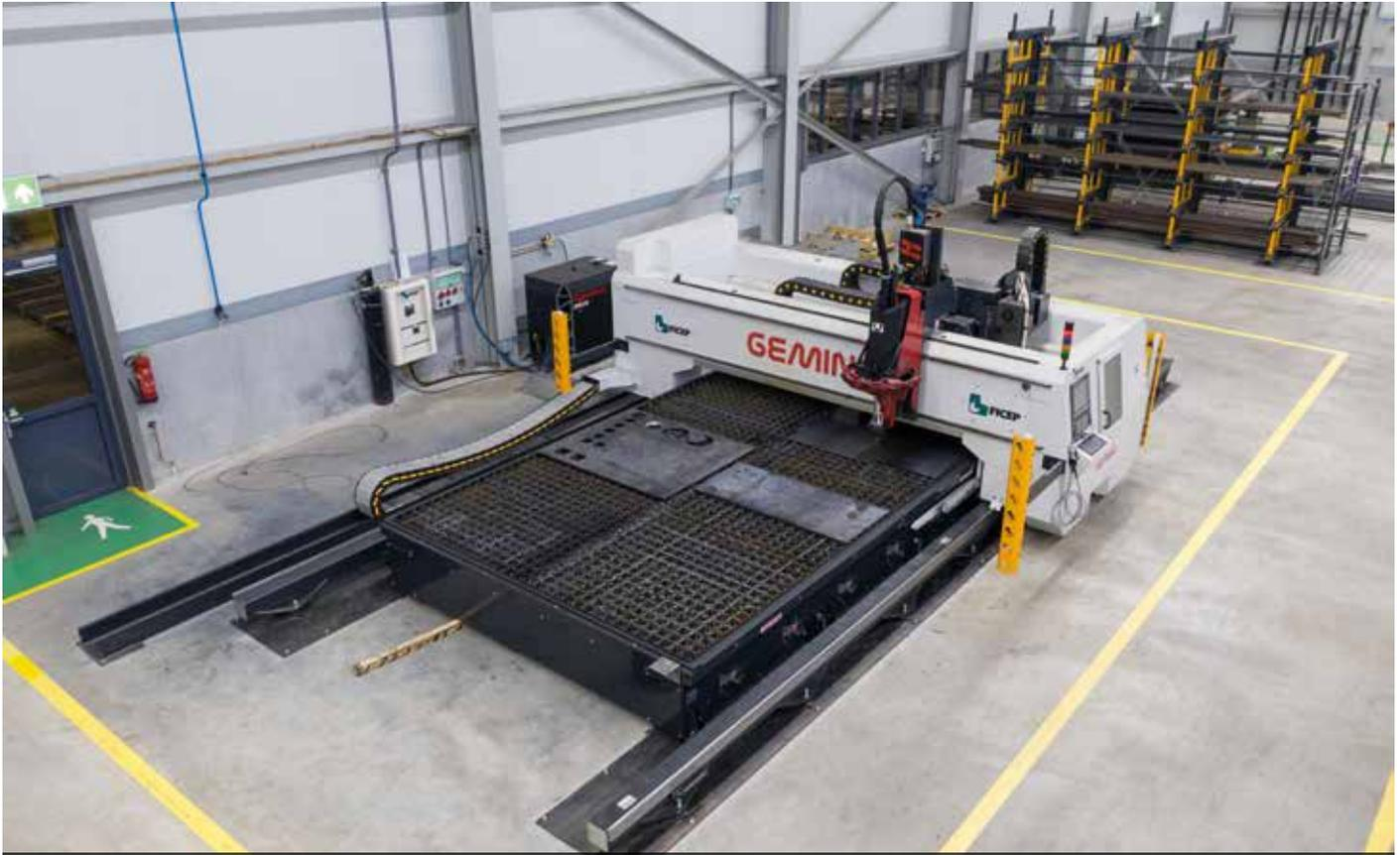
*FICEP GEMINI Gantry System for plate burning with plasma bevel head, drilling, milling and automatic plate layout*
