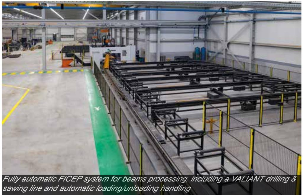
*Fully automatic FICEP system for beams processing, including a VALIANT drilling & sawing line and automatic loading/unloading handling*
