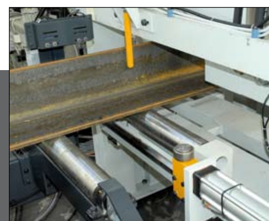
Horizontal and vertical clamp system to hold pieces during operations.
