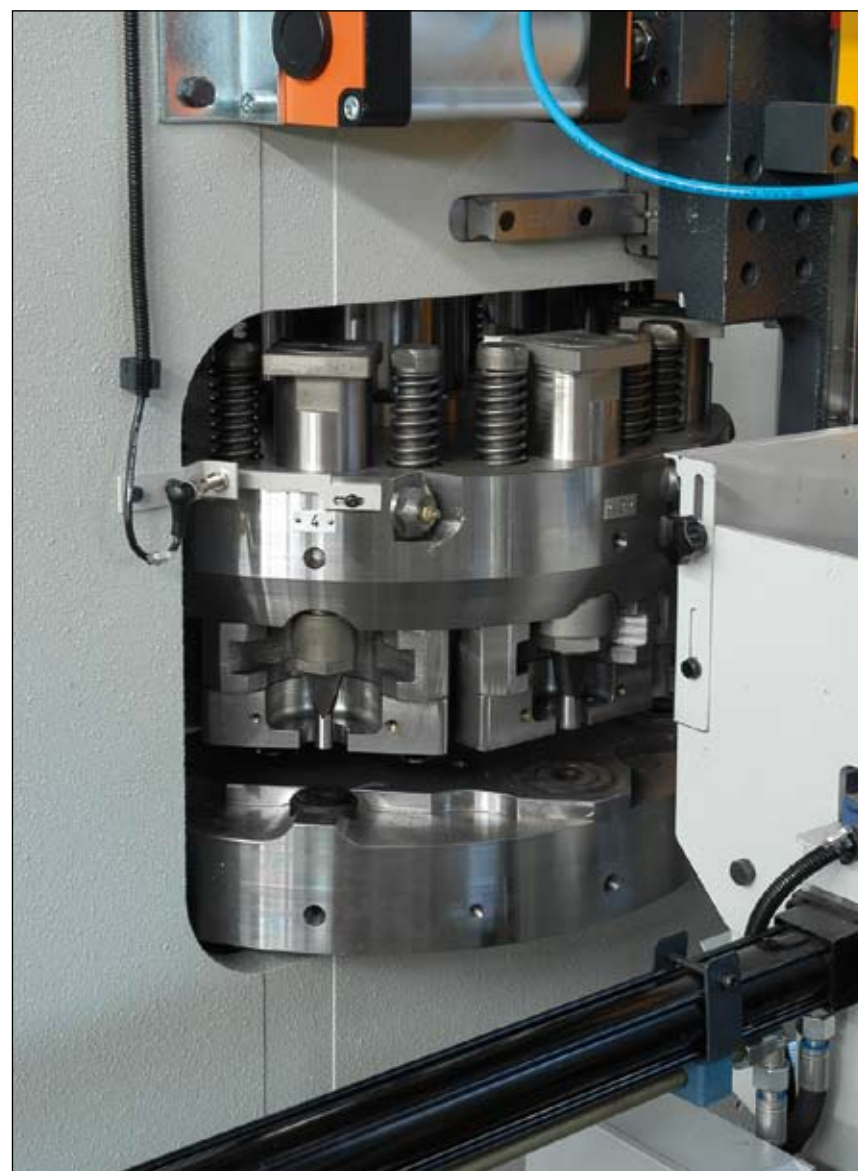
Tipo D8 punch for plates. 1100kN punching unit provided with automatic selection and rotation of 8 different punching diameters.
