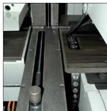
TIPO D4 optional 80 kN marking unit with 38 characters for pieces CNC controlled marking.
