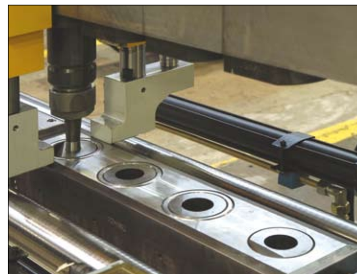
Tipo D4 punch for plates. 1100kN punching unit provided with four punches selected from the automatic program.
