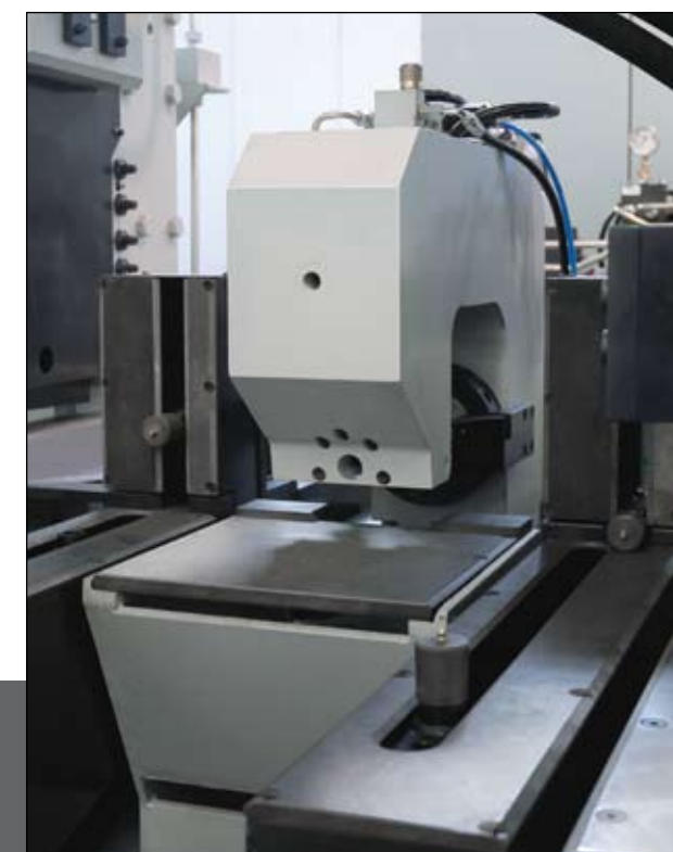
Punch for angle unit. Horizontal punching unit with 2 selectable punches for putting holes in the vertical flange of angles on any gauge line.
