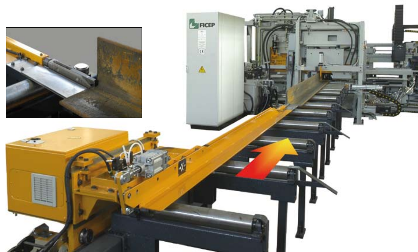
Horizontal and vertical clamp system to hold pieces during operations.
