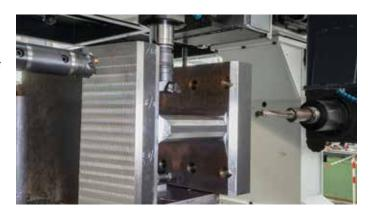
More often than not, holes in the flanges and the web do not share the same length coordinates as the web holes are generally skewed, for example, so each web hole has a different length coordinate. Even if holes share the same length coordinate in two of the surfaces, the girder is probably not positioned parallel to the travel of the gantry.
