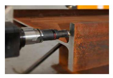
The web spindle of the FICEP girder gantry can also rotate up to 90° in each direction to be able to perform end milling.
