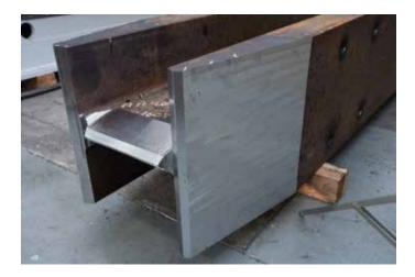
Since the girder is stationary and the spindles have their own independent sub axis, they can also perform the milling of weld preparation at aggressive rates as each spindle is driven by a 31 KW (41 HP) "Direct Drive" so the full motors power is what is being delivered to the tool.
