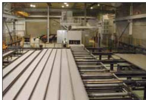
Through the installation of a cross feeding system, many efficiencies can be achieved. Also with a cross feeding system incorporated, the blasting machine can be integrated into a cutting/drilling line.
