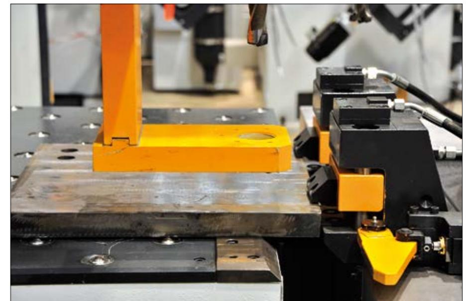
Vertical hold down and clamps
