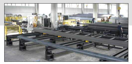
The lift and carry transfer systems by Ficep Corporation features multiple stands based upon the maximum and minimum section length that is to be conveyed. Each stand contains a chain driven material positioning cart. The material position cart is guided along a structural track and lifts hydraulically so the section can be positioned effortlessly and without objectionable noise to the next required location.
