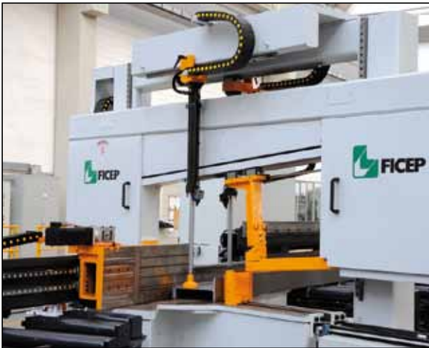
Automatic unloading device with magnet (optional)
