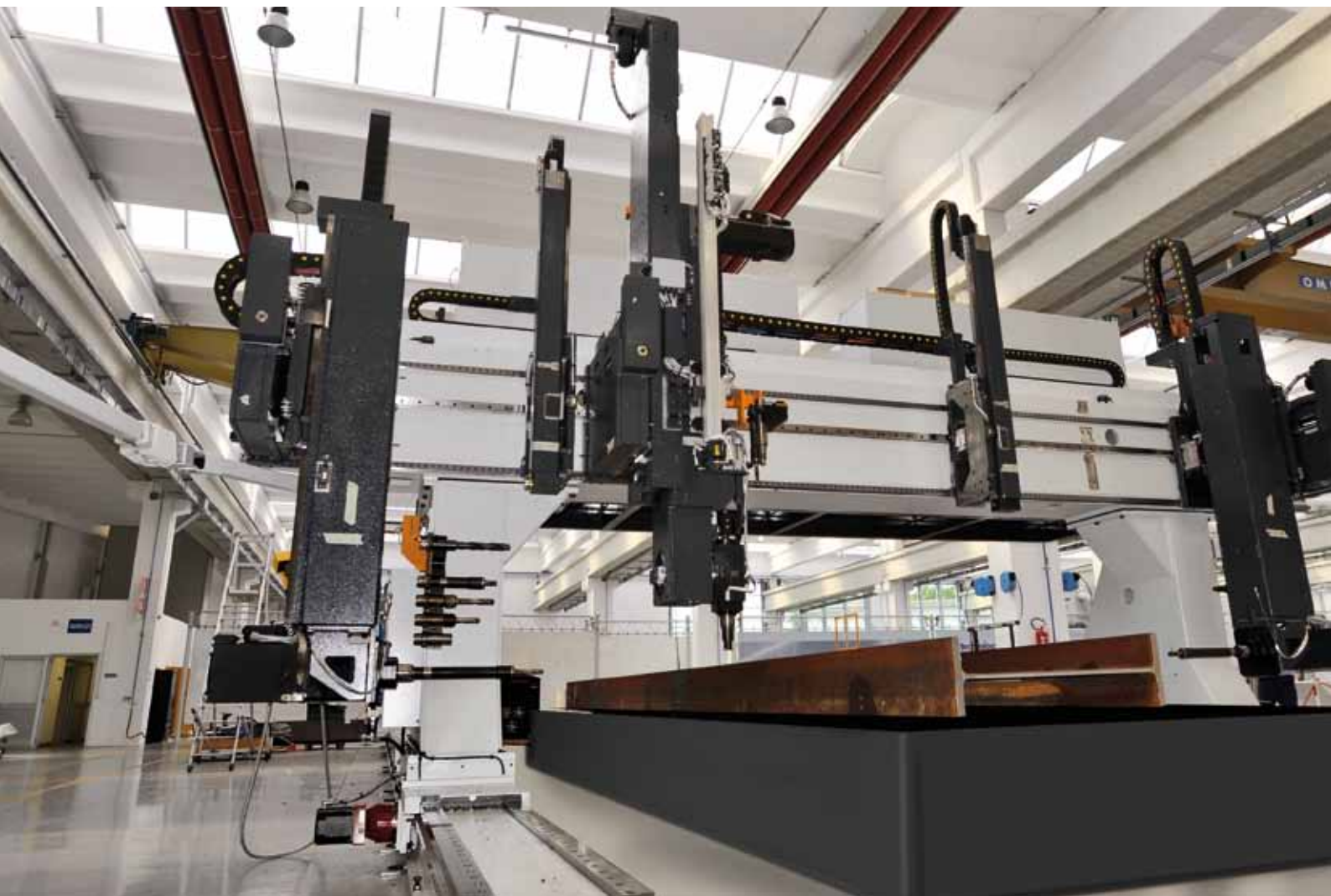
The largest drilling units in the Endeavour range are with a moving Gantry frame. These machines are ideal for e.g. large bridge girders.
