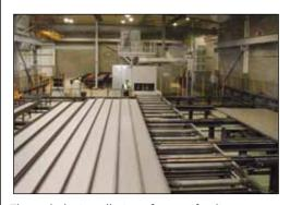
Through the installation of a cross feeding system, many efficiencies can be achieved. Also with a cross feeding system incorporated, the blasting machine can be integrated into a cutting/drilling line.
