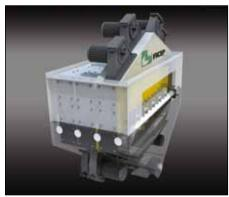
The shot blasting cabinet is manufactured completely from manganese. Manganese has a property which is hard enough to deal with the shot blasting from 35HRC to more than 50HRC. In the hot spot area of the blasting cabinet, additional 10mm thick manganese plates are added. They are attached from the outside and are easy to replace.
