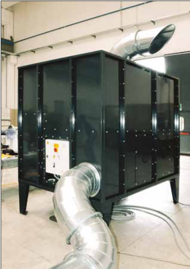
Exhaust system for Ficep plasma and/or oxycutting bench
