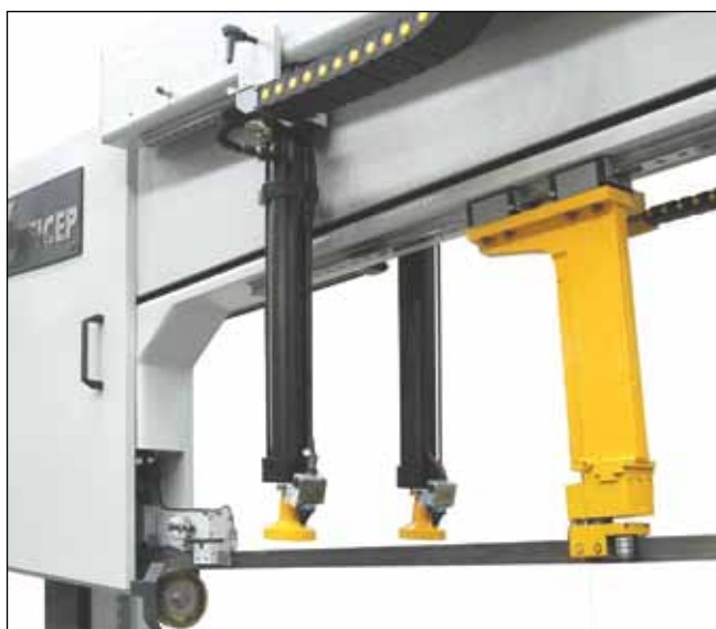
hydraulic vertical hold-downs that manually slide on prismatic guides
